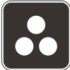
**Pump 2 Key:** Press this key once to turn Pump 2 onto Low speed, press this key a second time to turn Pump 2 onto High speed, a third press will turn the pump off. A built-in timer will shut the pump off after 20 minutes of operation unless done so manually. The Pump 2 Indicator will illuminate while the pump is running.
