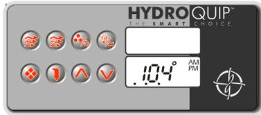
**Three Flashing Dots with Pump Off:** To prevent damage to your equipment, Hydro-Quip installs a pressure or flow switch. If 3 flashing dots appear below the temperature display while there is no pump(s) operating, turn the pump(s) on. If the 3 flashing dots went away this indicates that the pressure or flow switch was activated although there was no water flow.
