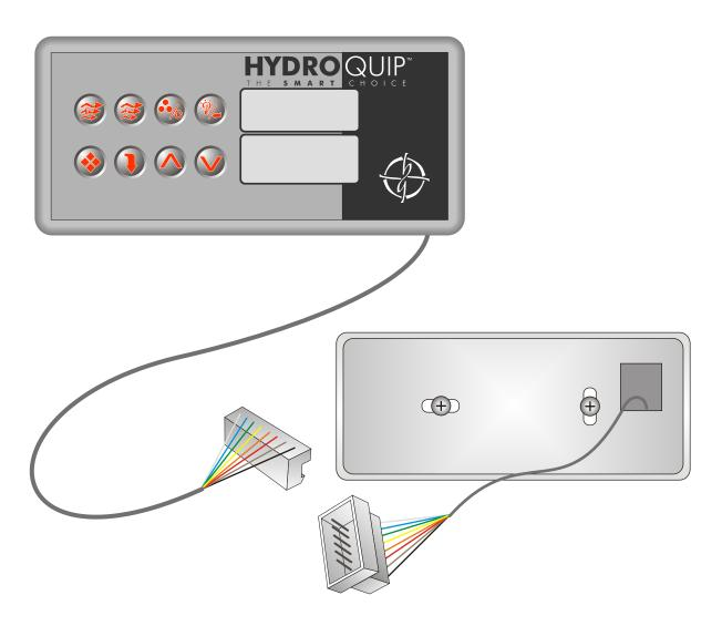
3 Connect the In-House Control female connector to the male cord-end connector as illustrated above.
